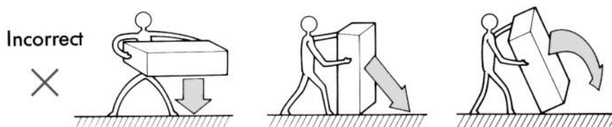
Fig. 2. Not Recommended Rolls Transportation
